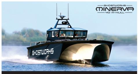
Minerva, built on our proprietary 14 Meter M-Hull platform, combines advanced carbon construction with cutting-edge design for exceptional speed, stability, and strength in unforgiving maritime environments. A low signature, reduced wake scar, and modular, subsystem-agnostic architecture enable rapid mission-specific configuration—ISR, defense, SAR—supporting crewed or fully autonomous operation.
